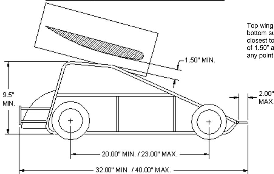
Top wing must be mounted so that the bottom surface of the top wing (point closest to the top of the cage) is a minimum of 1.50" above the roll cage and frame at any point, including downtubes.
